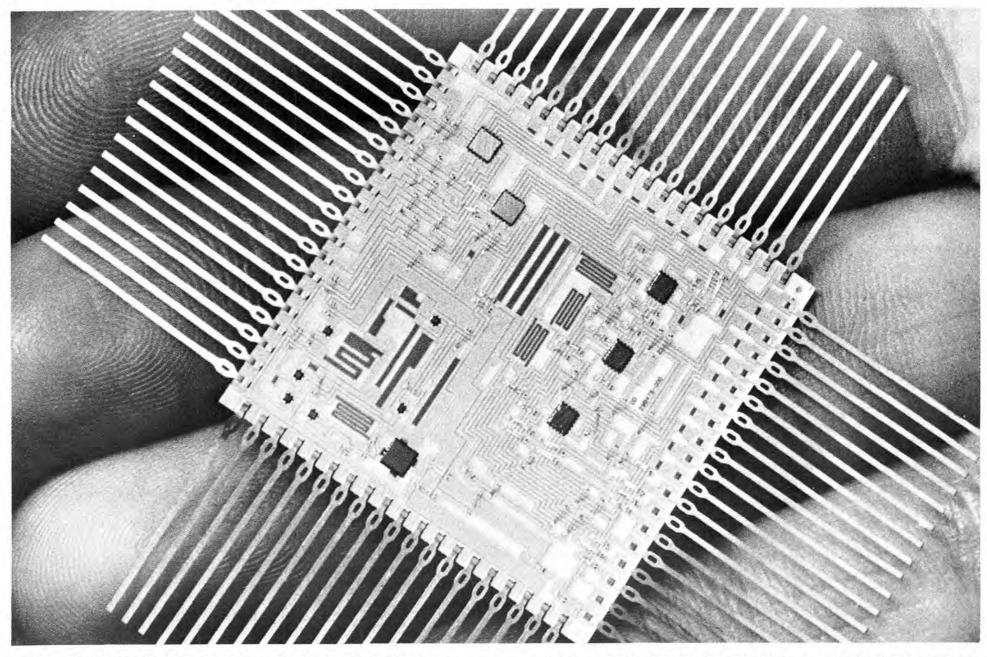
HYBRID CIRCUIT, enlarged here about four times normal size, reveals silicon integrated circuits (dark rectangles), transistors, capacitors, and diodes. Conductors and thin film resistors are formed directly on the substrates.
